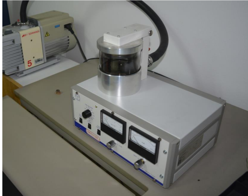
Figure 20. Gold and palladium sputter for the zirconia implants (SC7620 Mini Sputter Coater, Quorum Technologies Ltd, UK).
