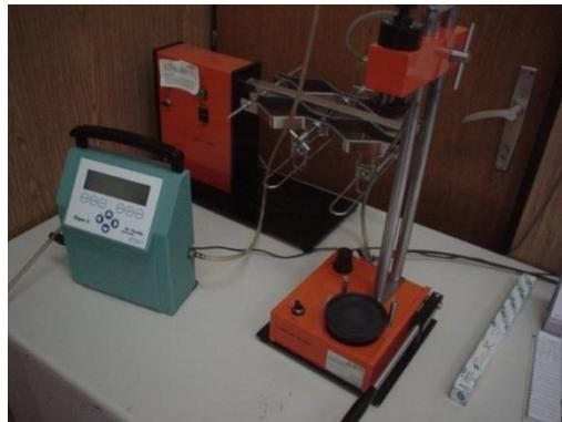
**Slika 45** Okretač boca BT-002, LG-automatic aps., Oksimetar Digox 5
