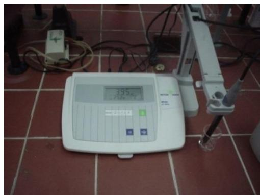
**Slika 35** pH metar MP220 (mv)
