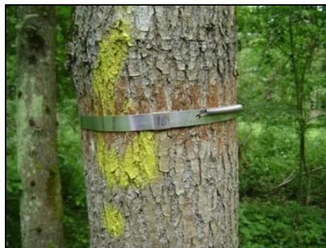
Figure 2.6: Tree with installed dendrometer band
