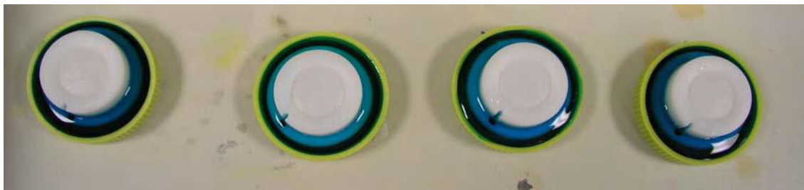
Figure 2.14. Pseudo DGT deployed in dye solution (Wagner, 2004).
