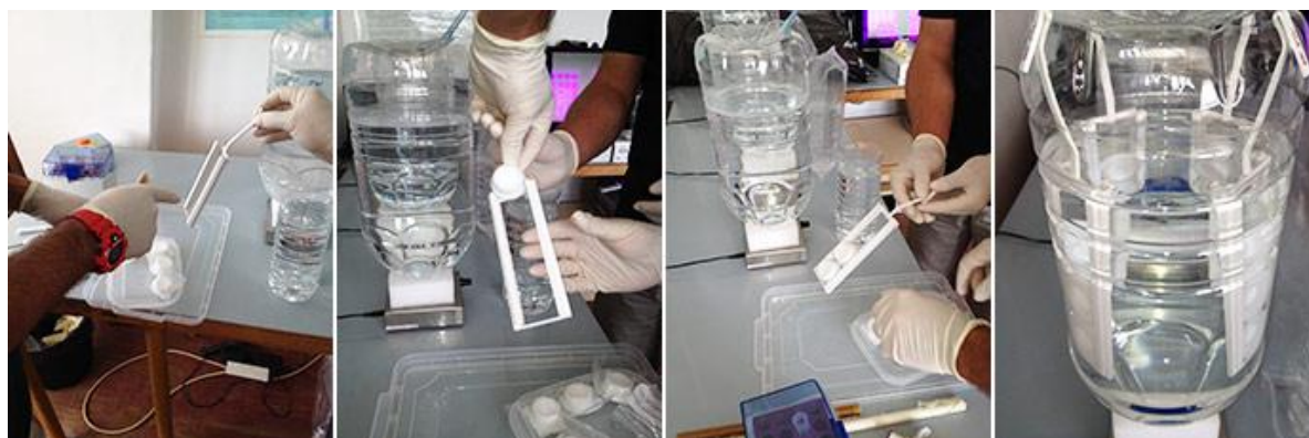
Figure 3.16. Set up for DGT “diffusion coefficient” experiment
