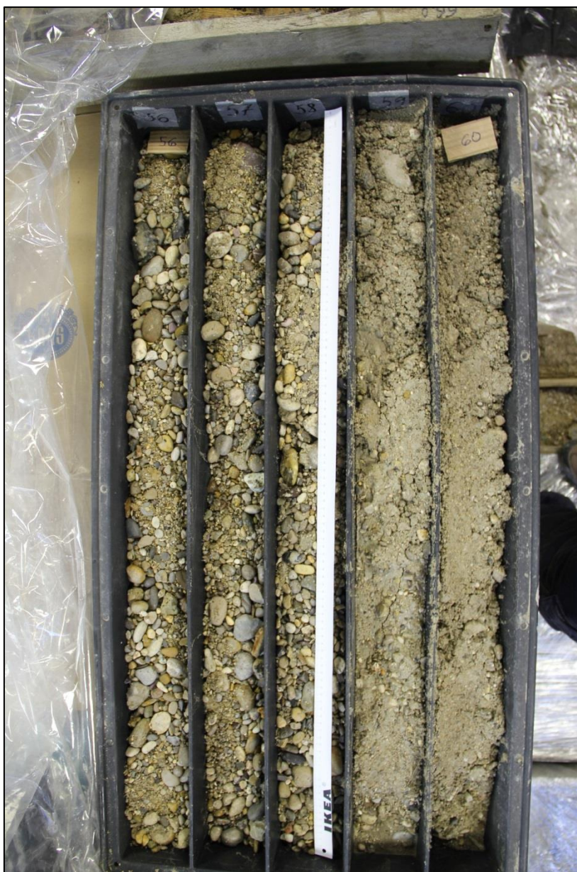
Figure 6.15. Sandy gravels and gravelly sands from the core NER120 (depth 56-60 m), interpreted as alluvial sands and gravels deposited during last glacial lowstand.
