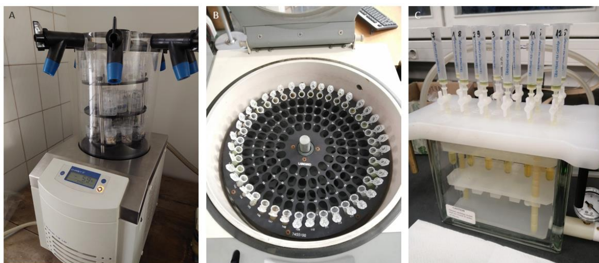
Figure 9. Sample processing. A) freeze drying of samples; B) drying supernatants in evaporator; C) purifying samples with Oasis HLB columns.
