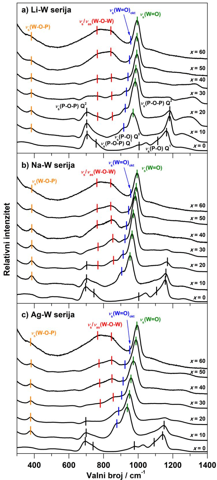
Slika 22. Ramanovi spektri svih stakala serija  $(30-x/2)\text{M}_2\text{O}-(30-x/2)\text{ZnO}-40\text{P}_2\text{O}_5-x\text{WO}_3$ ,  $x = 0-60$  mol%, M = Li, Na, Ag.
