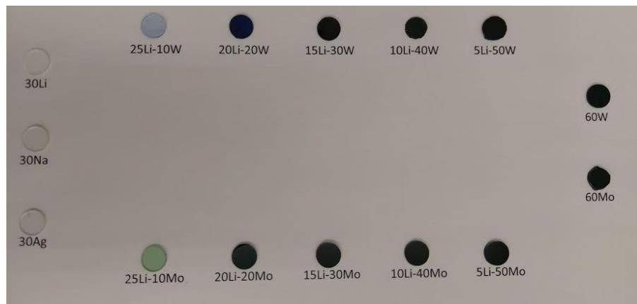
Slika 18. Fotografija priređenih uzoraka litijevih serija stakala, gornji red:  $(30-x/2)\text{Li}_2\text{O}-(30-x/2)\text{ZnO}-40\text{P}_2\text{O}_5-x\text{WO}_3$ ,  $x = 0-60$  mol%; donji red:  $(30-x/2)\text{Li}_2\text{O}-(30-x/2)\text{ZnO}-40\text{P}_2\text{O}_5-x\text{MoO}_3$ ,  $x = 0-60$  mol%.
