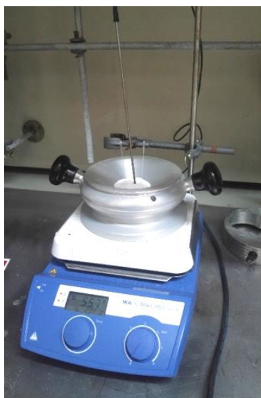
Figure 50. Experimental setup for the crystallization of high temperature NaIm polymorph in the form of the single crystal.
