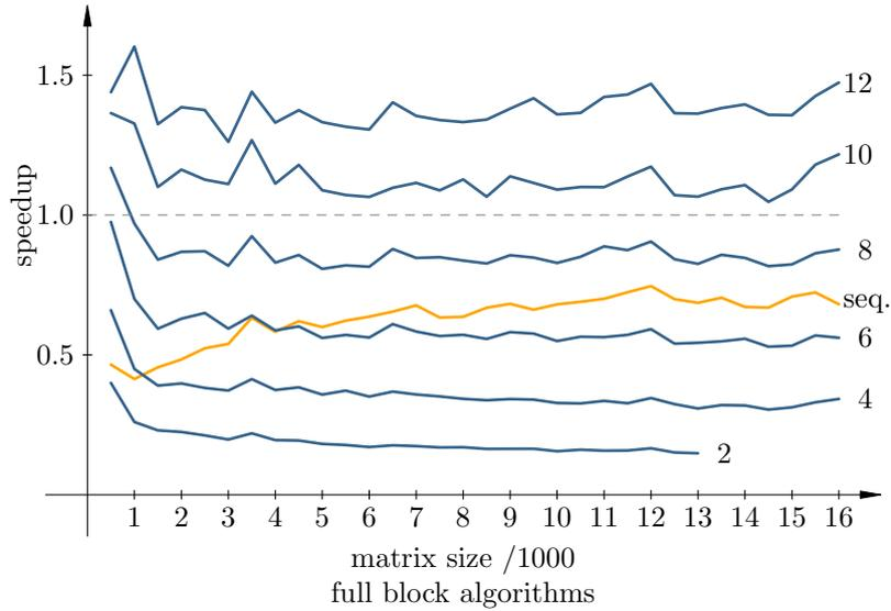
Figure 3.4: Speedup of the shared memory full block algorithm on 2–12 cores vs. the sequential block-oriented Hari–Zimmermann algorithm (with MKL threaded on 12 cores). An additional curve (denoted by seq.) shows the “speedup” of the sequential full block algorithm vs. the block-oriented algorithm. A few missing values for 2 cores are caused by the limit of execution time on the cluster (12 hours).
