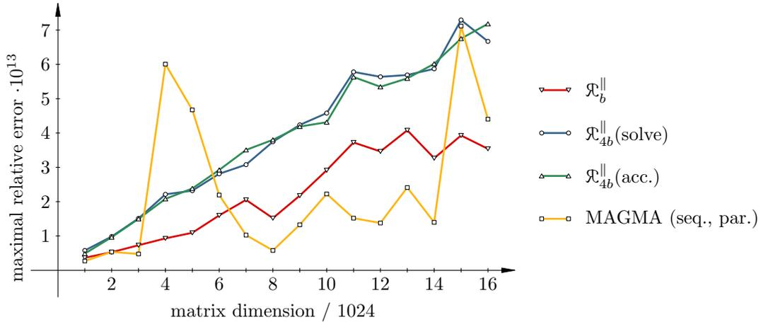
Figure 2.26: The relative accuracy of the block-oriented 1- and 4-GPU Fermi implementations and MAGMA. The test spectra are  $\Lambda_k^{(2)}$ .
