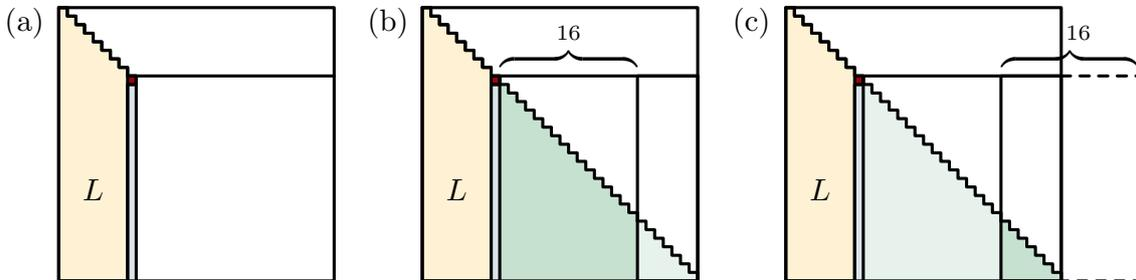
Figure 2.10: The forward-looking Cholesky factorization  $H_{pq} = L_{pq}L_{pq}^T$ .
