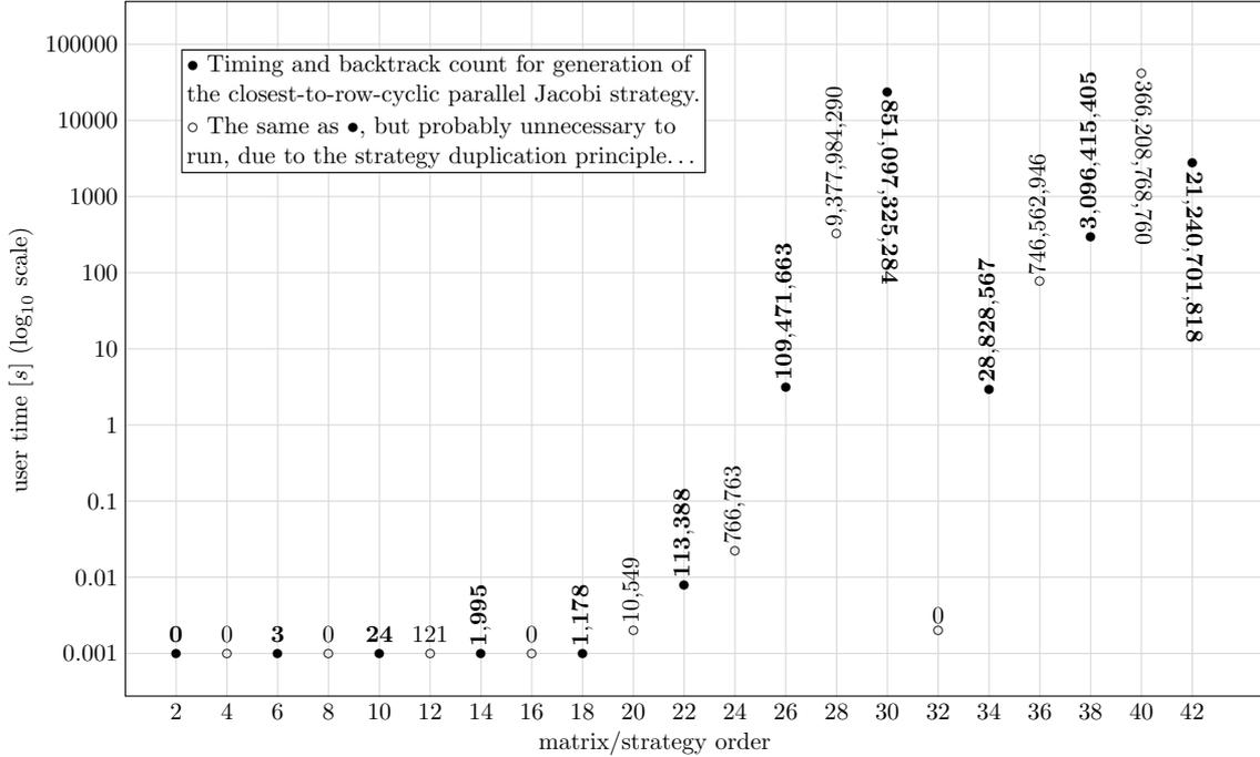
Figure 2.9: The user part of the execution time, as reported by `time` utility, of  $\mathcal{R}^{\parallel}$  generation, with a number of pivot candidates discarded (i.e., the algorithm’s “backtracks” counted as in Listing 1) per each strategy/matrix order, on an Intel Core i5-4570 CPU @ 3.20GHz with `clang-703.0.31` C++ compiler (macOS Sierra).
