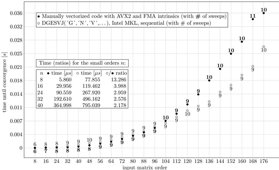
Figure 4.1: Execution times and sweep counts of the manually vectorized Jacobi code with AVX2 and FMA intrinsics, vs. `DGESVJ` from Intel MKL 2017.2.163 (sequential), on Intel Core i7-4850HQ CPU @ 2.30GHz, with macOS 10.12.4 and `clang-802.0.38`. Measured with `CLOCK_THREAD_CPUTIME_ID` POSIX clock, per run, and averaged over 100 runs; see <https://github.com/venovako/JACSD/tree/master/test> for more.
