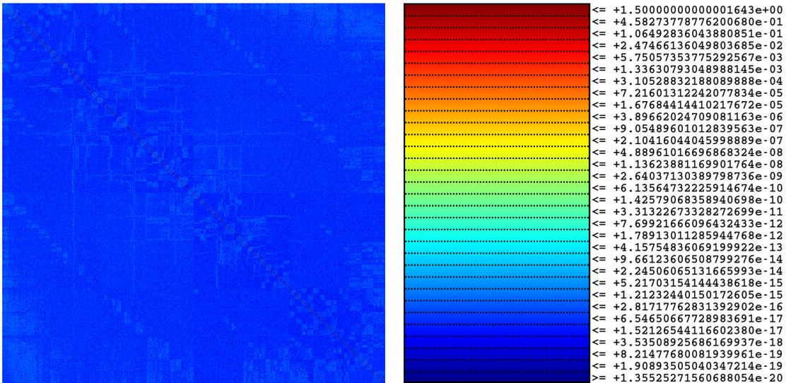
Figure 2.17:  $|G^T G|$  after block-sweep 8. The heatmap corresponding to  $|G^T G|$  after the last (9<sup>th</sup>) block-sweep is omitted because it is hardly distinguishable from the one for the 8<sup>th</sup> block-sweep. A colorbar, with the value ranges for  $|G^T G|$  in  $\log_2$  scale, is shown instead.
