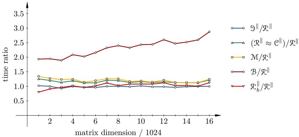
Figure 2.21: The wall-clock time ratio of the various parallel strategies on a single GPU (Fermi). The test spectra are  $\Lambda_k^{(1)}$ .
