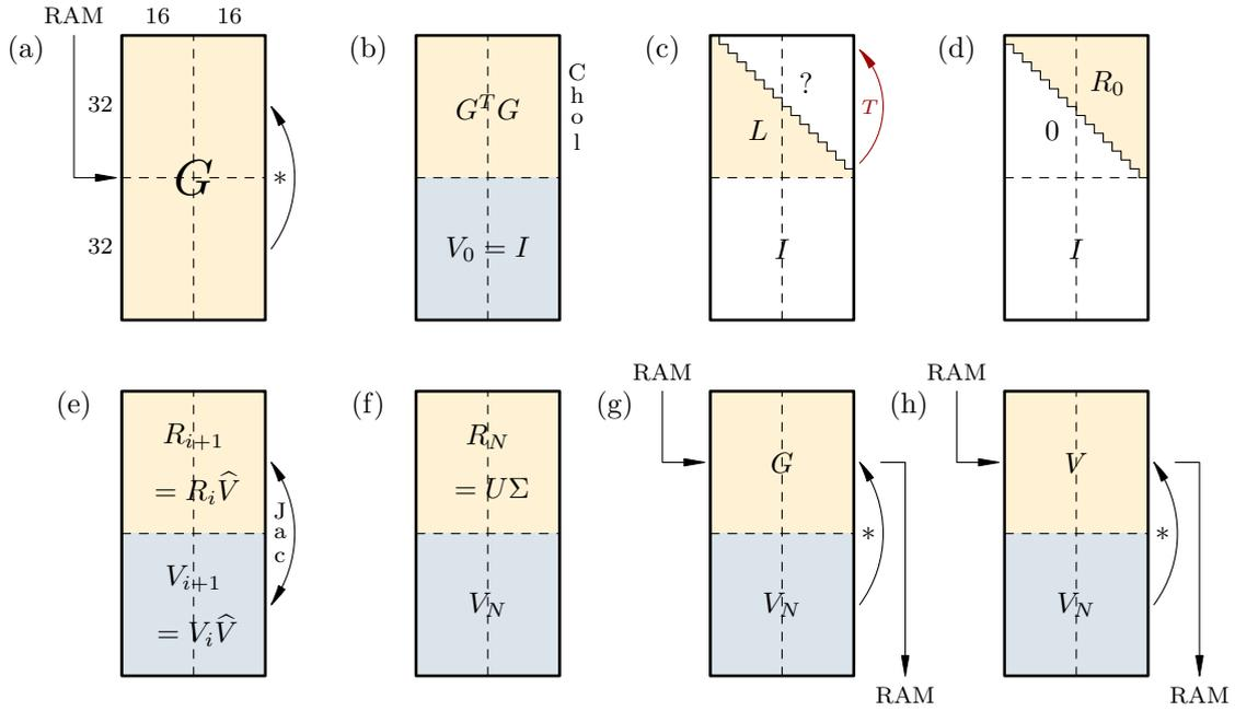
Figure 2.12: An overview of `pStep` kernel per thread block, the full block variant. Each subfigure depicts the state of the shared memory, the computation subphase performed, and the data transfer in or out of the GPU RAM. Subfigures (a)–(d) illustrate `factorize` with the Cholesky factorization, (e) and (f) belong to `orthogonalize`, and (g) and (h) to `postmultiply` phase.
