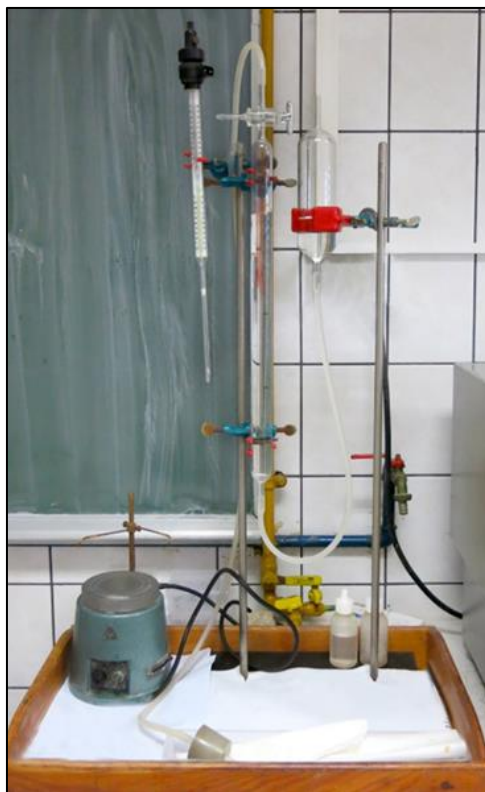
Figure 4.7. Calcimeter for determination of carbonate share in samples (Division for Mineralogy and Petrology, Department of Geology, Faculty of Science, Zagreb).
