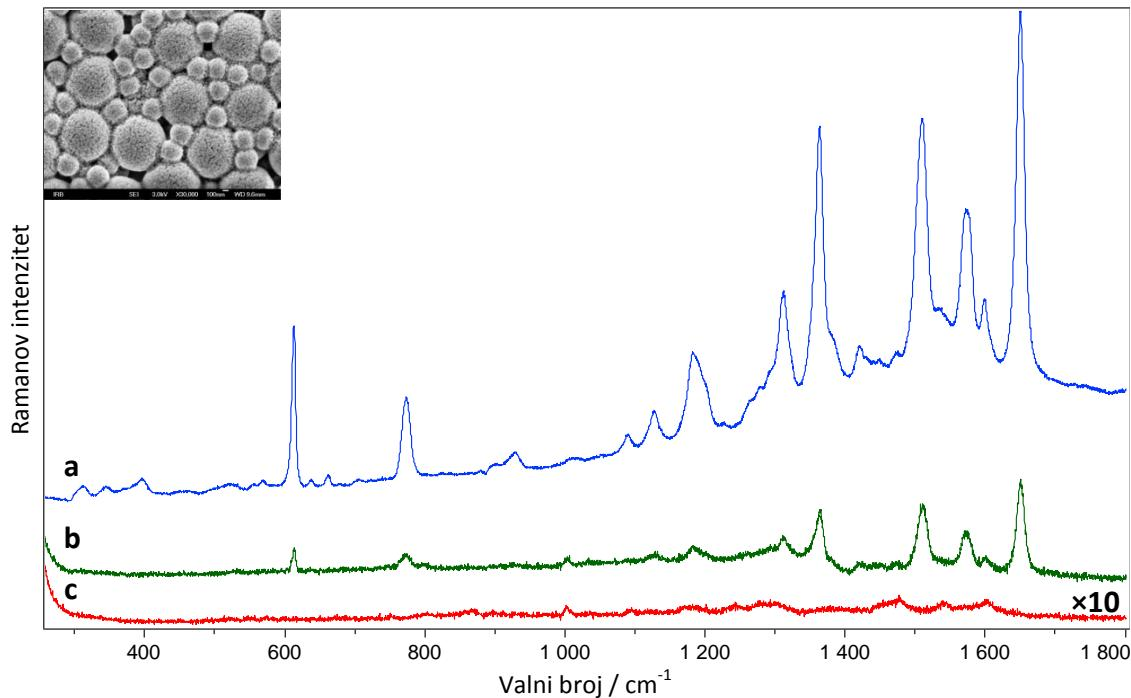
Slika 85 SERS spektri R6G na uzorku 80 nm / (350 nm + 1000 nm): a)  $10^{-6}$  M, b)  $10^{-8}$  M i  $10^{-9}$  M ( $\lambda=514,5$  nm; 0,5 mW; vrijeme snimanja 30 s; 100 x).
