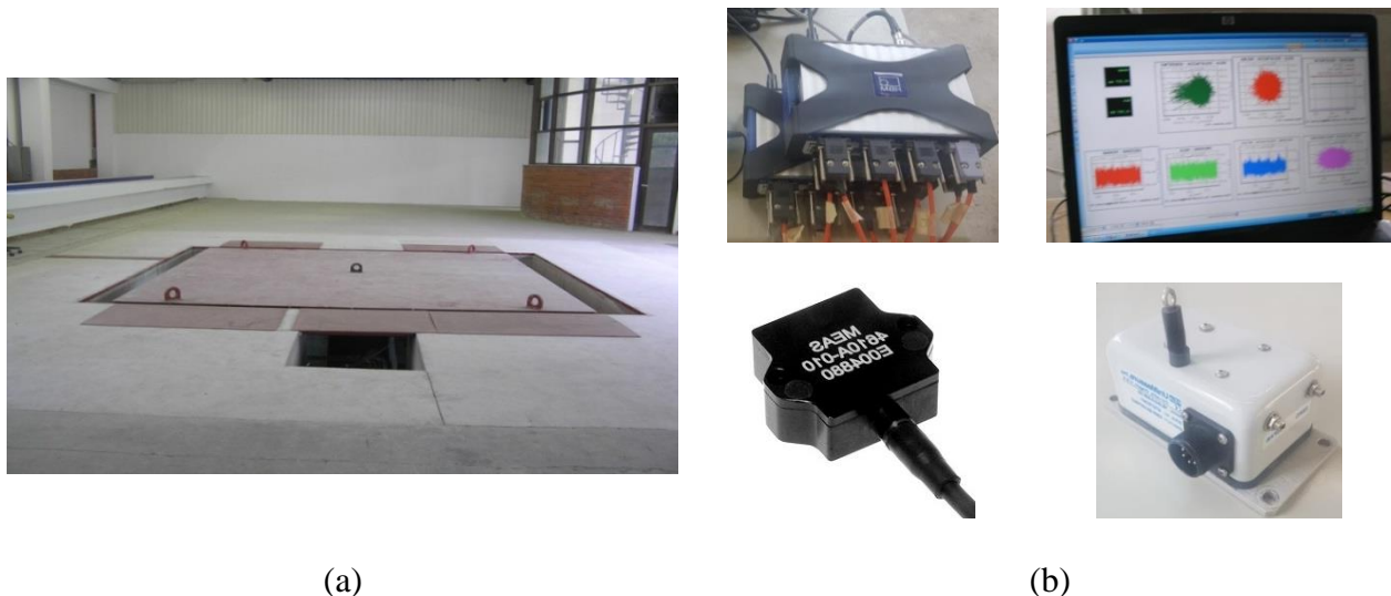
Figure 2.11 Test equipment: (a) Uniaxial shake-table; (b) Data acquisition system and some sensors for measuring mechanical values
