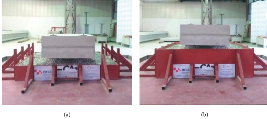
FIGURE 9: Photos of experimental setup before testing. (a) Pebble layer h_p = 0.3 m. (b) Pebble layer h_p = 0.6 m.
