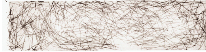
Figure 4.18: X-ray image of a fiber-reinforced concrete specimen [68].
