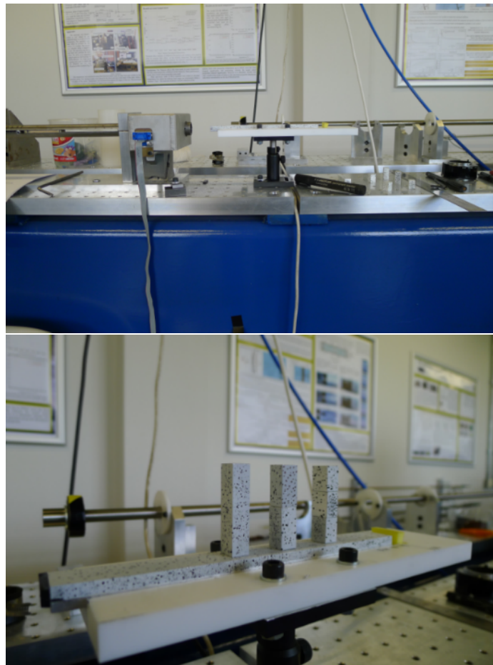
Figure 8.2: Optical bench and ROORI1 test facility (top); samples of multi-block structures on the sliding base (bottom)
