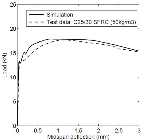
(c) model s udjelom vlakana od  $75 \text{ kg/m}^3$  betona ( $V_f=0.975\%$ )
