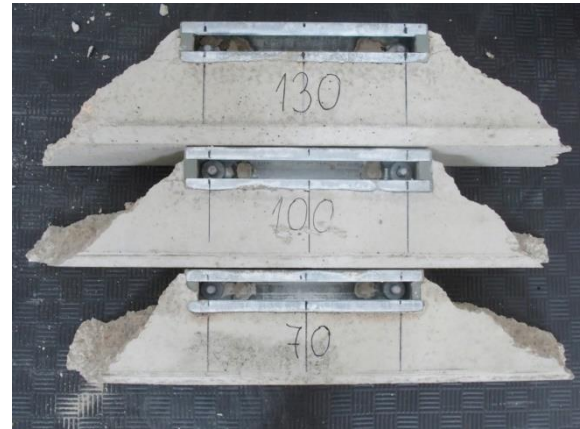
Figure 4.5 (a) Test results compared with the proposal and the current code provisions; (b) Top view of the breakout bodies for investigated member thicknesses (from above) of 130, 100 and 70 mm
