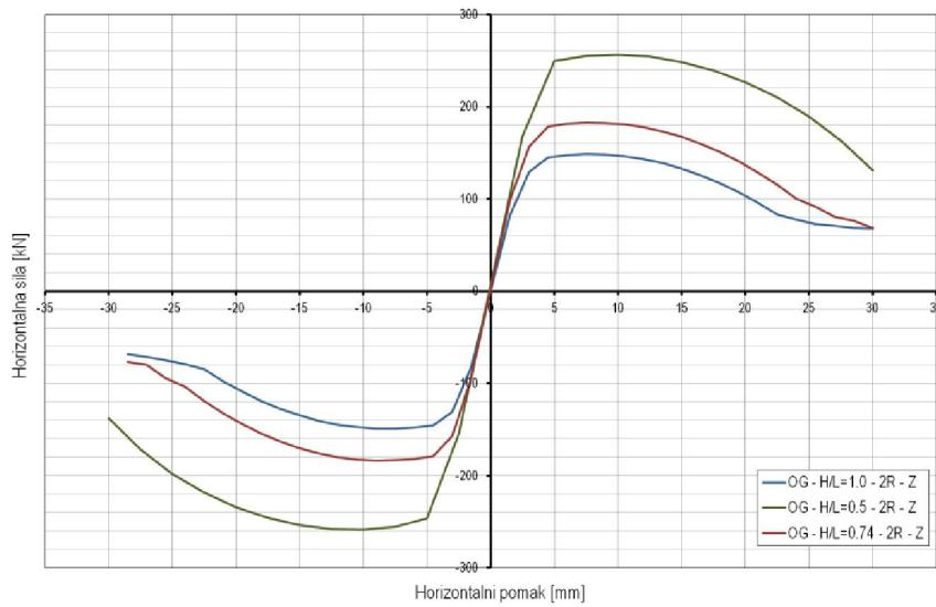
b) Zglobni priključak (Z) –  $H/L=0.50, 0.74, 1.0; R=2$
