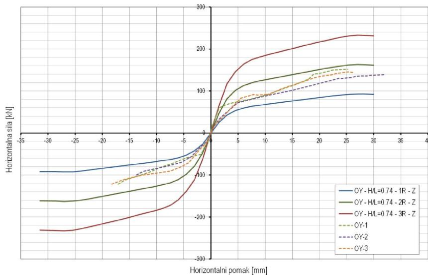
b) Zglobni priključak (Z) –  $H/L=0.74$ ;  $R=1, 2$  i  $3$
