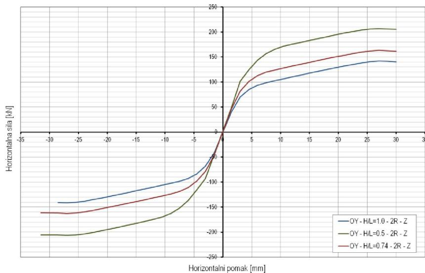
b) Zglobni priključak (Z) –  $H/L=0.50, 0.74, 1.0; R=2$
