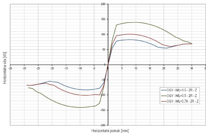
b) Zglobni priključak (Z) –  $H/L=0.50, 0.74, 1.0; R=2$
