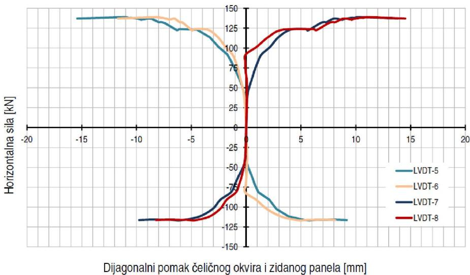
**Slika 4.43 – Pomaci dijagonalala – okvir OG-2**
