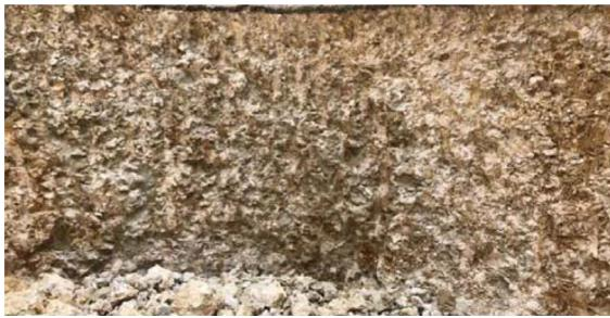
**Fig. 1** Weathered Simsima limestone layer
