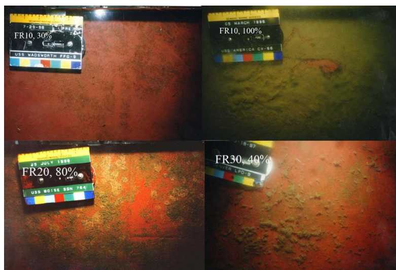
Figure 1.2 Fouling rating scale for soft fouling [40]
