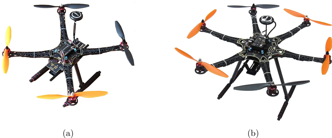
Figure 2.1: Multirotor types: quadrotor [89] (a), hexarotor [90] (b)
