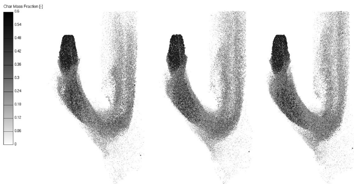
Figure 6. Char mass fraction in particles: Case 1 (left); Case 2 (middle); Case 3 (right).
