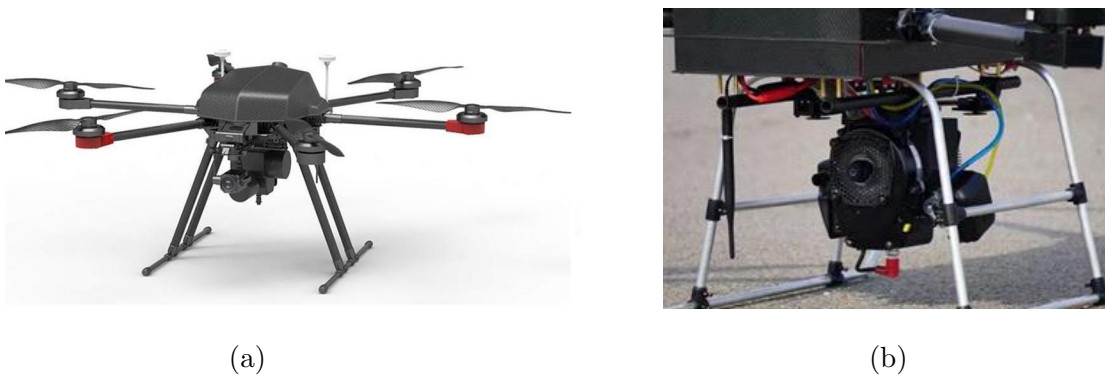
Figure 2.18: Walkera QL1200 [121] (a), H2 hybrid power unit for multirotors [122] (b)
