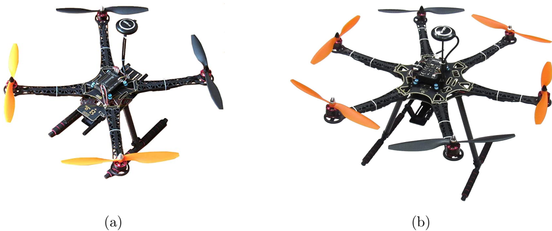
Figure 2.1: Multirotor types: quadrotor [89] (a), hexarotor [90] (b)
