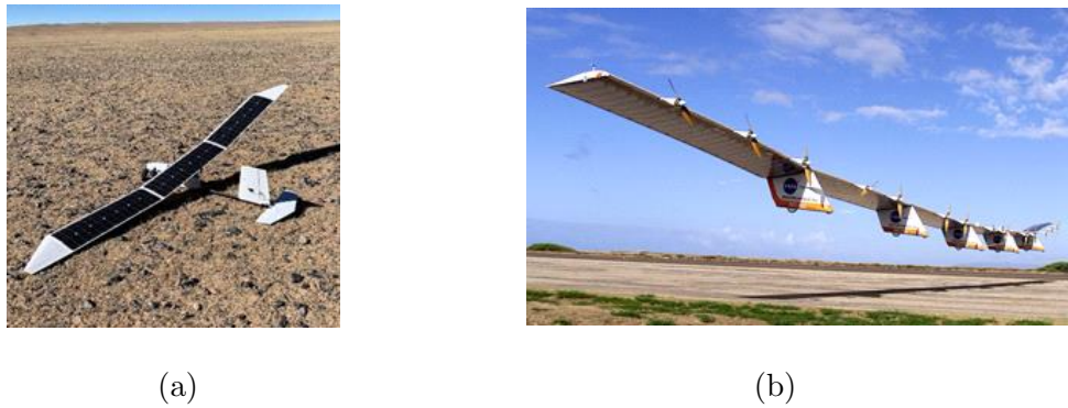
Figure 2.17: Small hand-launched solar-powered UAV [119] (a), Helios by NASA Prototype, ultra-lightweight flying wing [120] (b)
