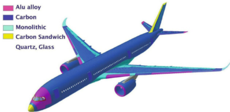
Figure 1.2: Airbus A350 structural materials [McConnell, 2011].
