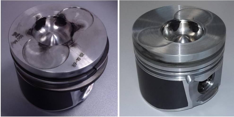
Figure 20. Left: original piston; right: after machining (-0.7 mm)
