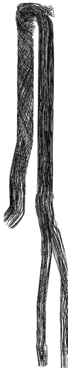
Fig. 2. Flow streamlines inside the calculated calciner.
