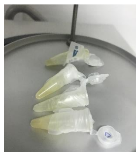
Figure 63 Removal of acetic acid from the CDHA sample by diluting the CDHA sample obtained after evaporation. CDHA lyophilization in 1.5 mL-locking microcentrifuges.
