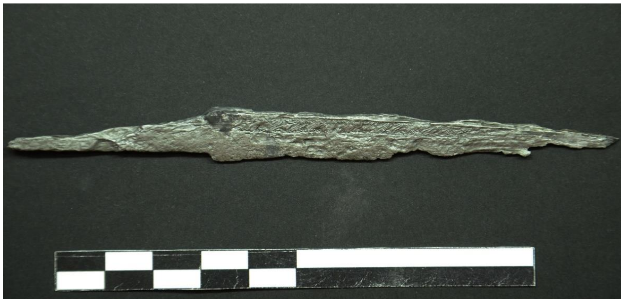
Photo 1-Pattern welded knife from Kobilić 1 (photo by Borko Rožanković)
