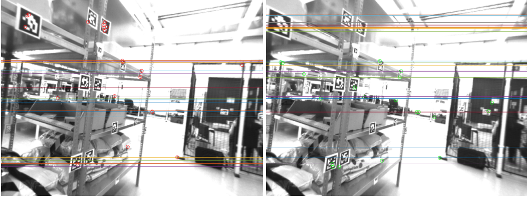
(b) Epipolar lines after rectification.
