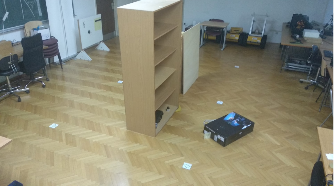
Figure 5.7: A setup for localization experiments with moving UWB anchors. Two moving UWB anchors are placed on the boxes which simulate moving robots.
