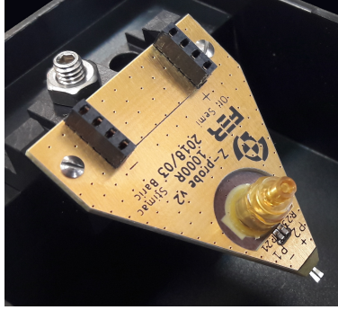
(a) Floating-ground probe design (top).
