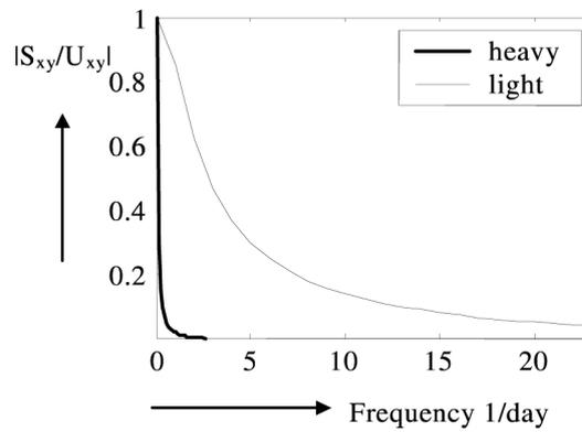
FIGURE 2.8. Cyclic transmittance for different walls, L[49]
