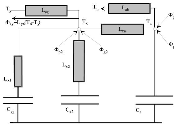
FIGURE 2.10. An indoor thermal model of admittance, L[49]
