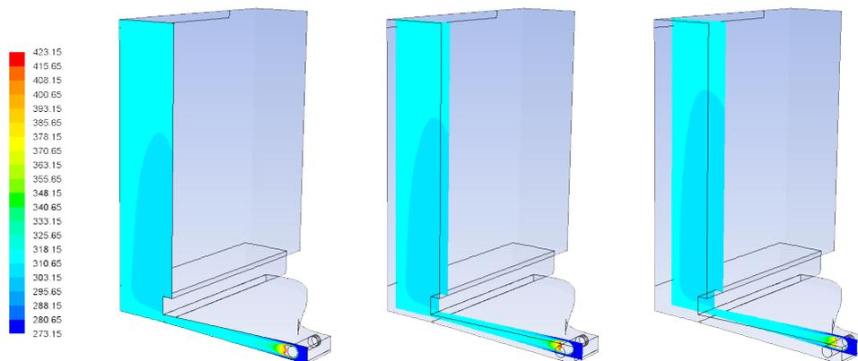
FIGURE 2.15. Temperatures [K] at  $y = \{0, 10, 20\}$  mm
