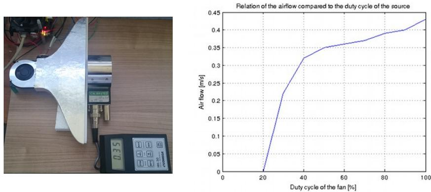
FIGURE 2.28. Air speed measurements a) Sensor position for measurement
