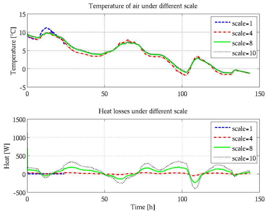
FIGURE 4.3. Influence of dimension variance in scale to air temperature in the zone
