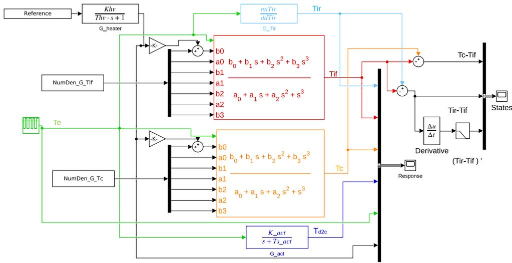
FIGURE 4.7. Block diagram of the improved model presented in *Simulink*
