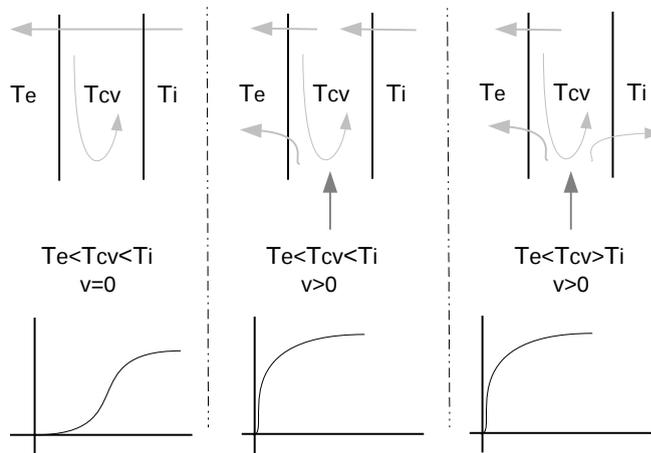
FIGURE 2.12. Heat flux directions in different DSF's work regimes
