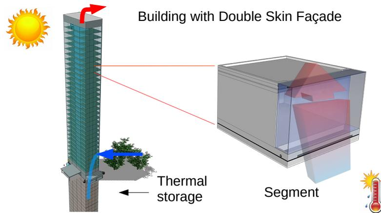
FIGURE 2.6. Segment of building with DSF
