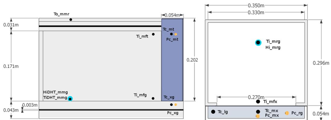
FIGURE 2.26. Dimensions with marked location for sensor deployment a) side view
