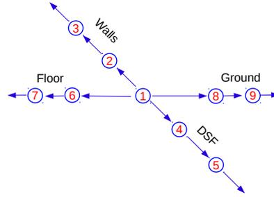
FIGURE 2.52. Thermal graph representation of the building segment
