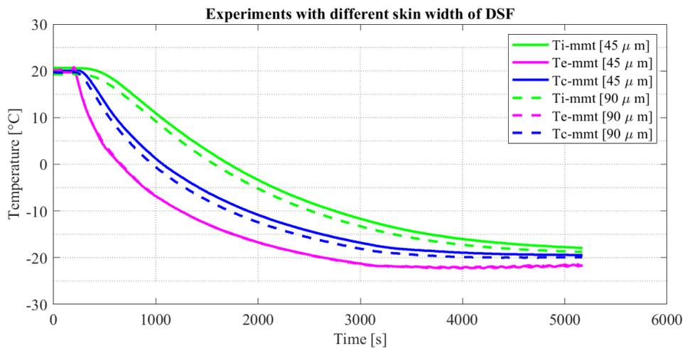
FIGURE 2.44. Temperature responses of the scaled mock-up with various plastic DSF
