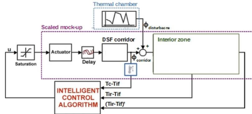
FIGURE 3.4. Block diagram of DSF control
