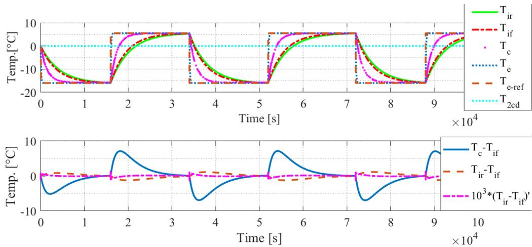
FIGURE 4.8. Simulated temperature responses of the scaled mock-up
