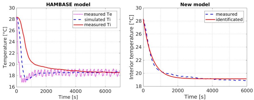
FIGURE 2.48. Interior temperature response of the scaled mock-up to external temperature step change a) HAMBASE model b) improved model
