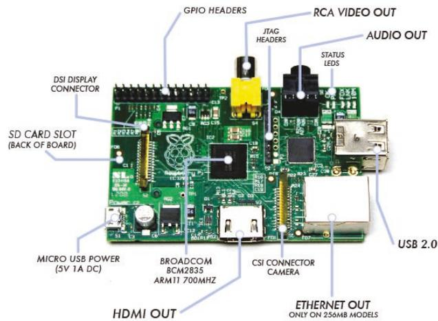
FIGURE 2.24. Low cost single board computer - Raspberry Pi
