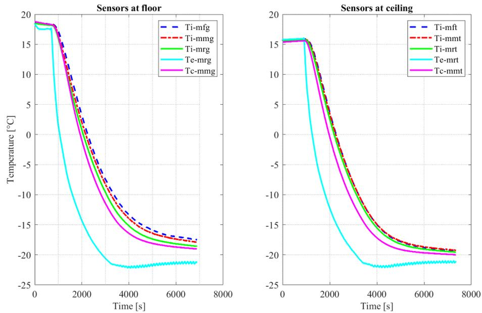
FIGURE 2.42. Temperature responses of the scaled mock-up with 1 cm wide DSF corridor: different vertical positions of the sensors
