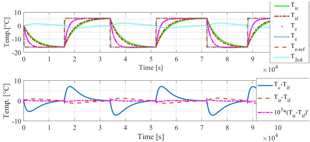
FIGURE 4.9. Simulated temperature responses of scaled mock-up with P regulator
