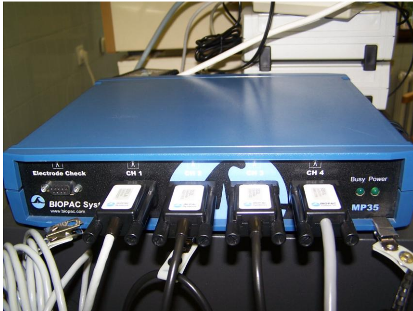
Figure 8.1. Biopac MP35 biopotential amplifier
