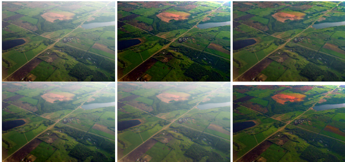
Figure 6.3: Top left is the original image, top middle image dehazed using VarDCP, and top right using Unsupervised DCP. Bottom left is dehazed using FFANet, bottom middle using Dehazeformer, and bottom right using DCP. FFANet and Dehazeformer barely affect the image at all. The DCP removes most of the haze, but the resulting contrast of the colors is a lot too high and look slightly unnatural. The same is true to a lesser extent for the VarDCP method. The Unsupervised DCP method produces the most natural-looking image in this case.
