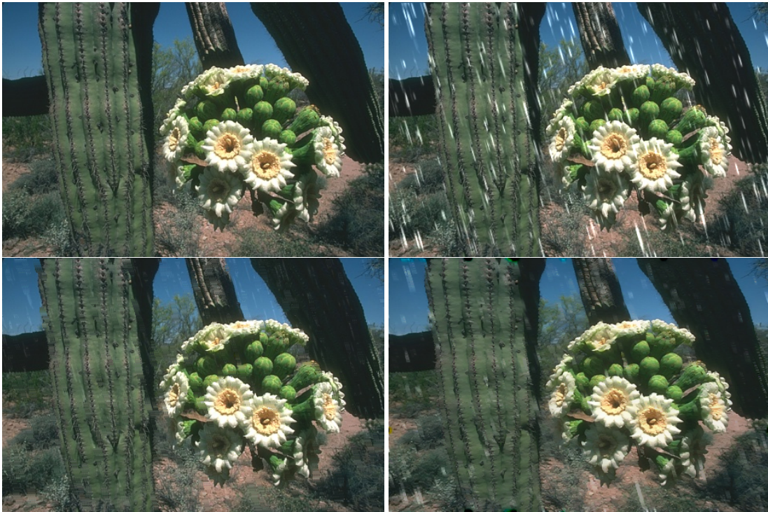
Figure 6.11: Top left is the ground truth rain-free image, top right is the image with added rain, bottom left is the version made with the proposed method using optimal W , and bottom right is the version derained with W = 1 everywhere. We can see that the rain is better removed, and other parts of the image are better preserved.
