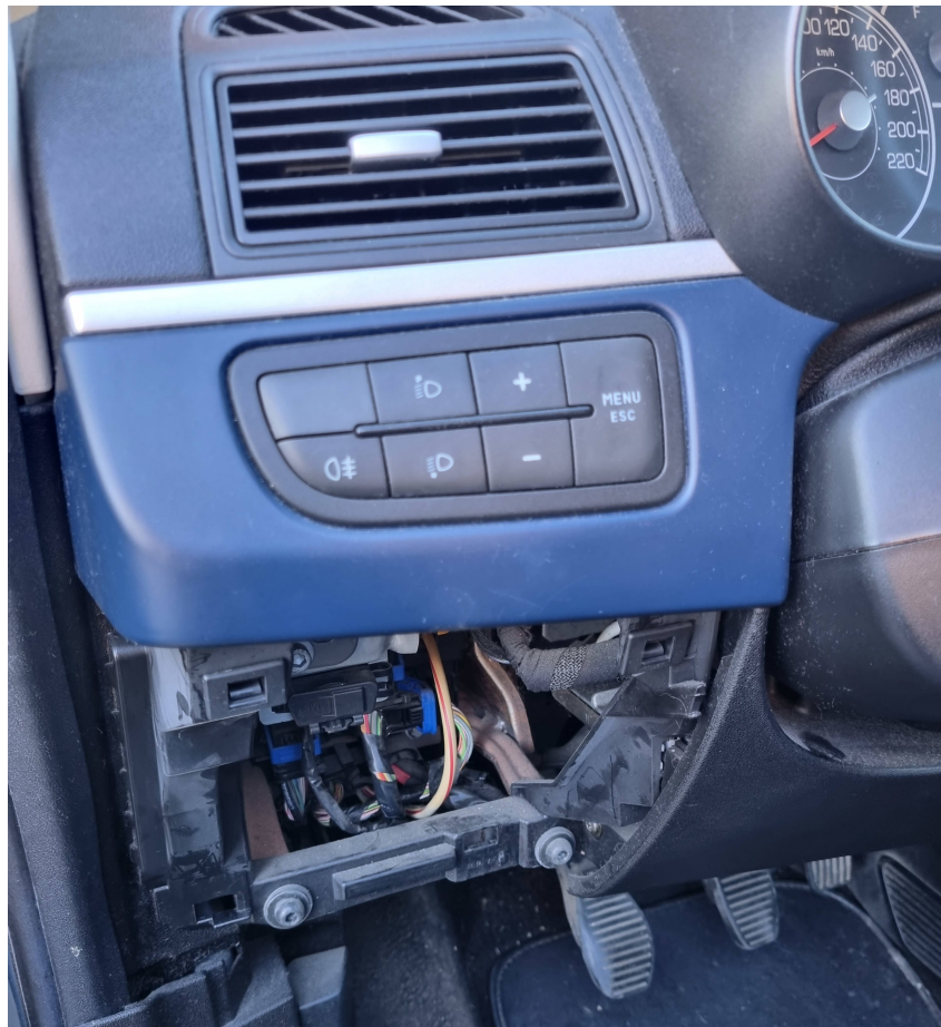
Figure 6.1: OBD-II port location in Fiat Grande Punto 2007
