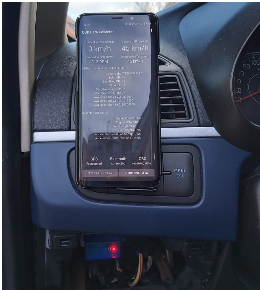
Figure 3.12: Automotive data collector application collecting automotive data via ELM-327 Bluetooth device
