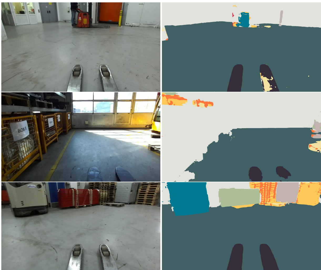
Figure 5.5: Examples of input images (left) and corresponding semantic segmentation on the RoMb dataset (right).
