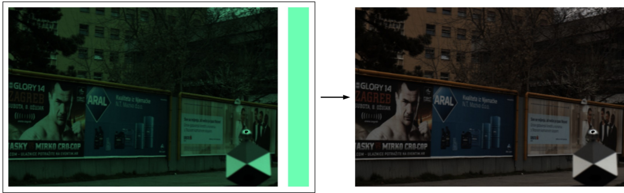
Figure 2.3: An example of applying von Kries-based chromatic adaptation model [10, 11]. Left: original color-biased image and the corresponding illumination color; right: corrected image is shown.
