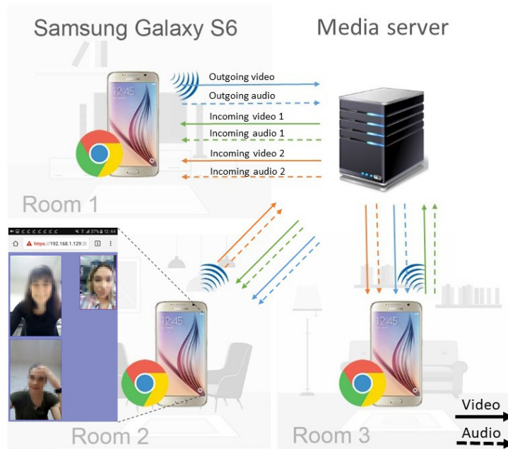
Figure 6.8: Testbed set-up over a LAN (user study US4).
