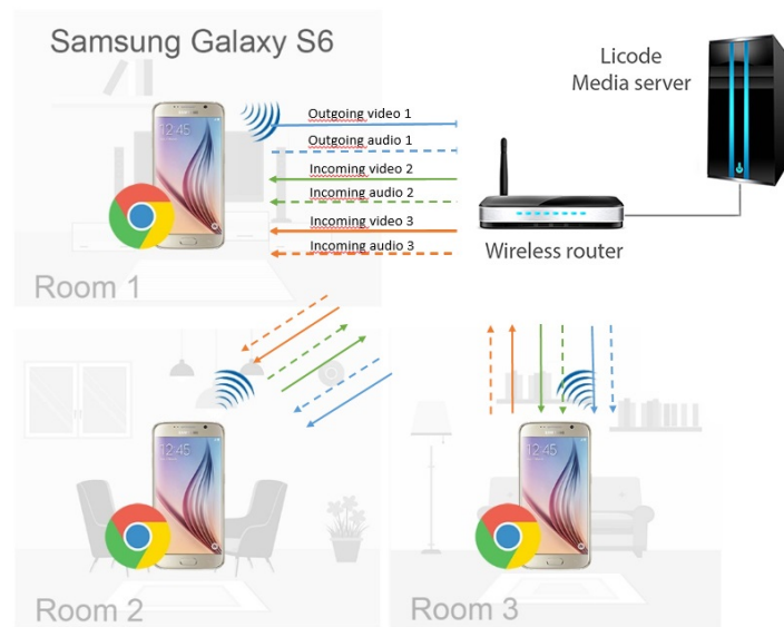
Figure 5.7: System set-up over LAN with Licode media server and Samsung Galaxy S6 (user study US2).
