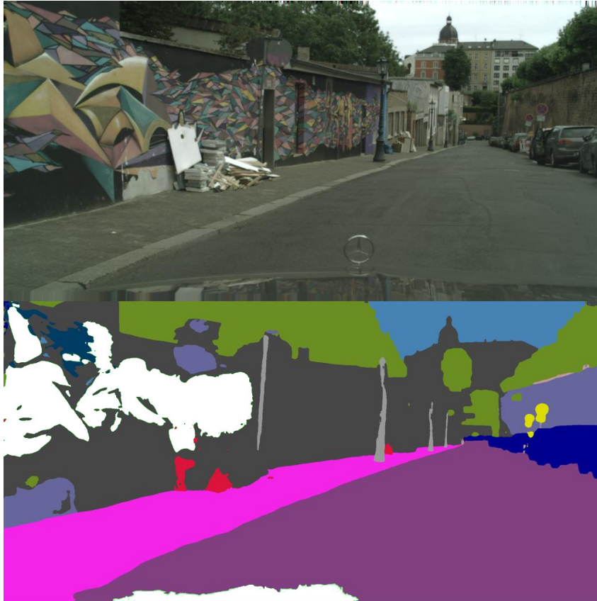
Figure 5.1: The only Cityscapes test image in which a large group of pixels was misclassified into indoor classes. The graffiti on the building (white pixels) were classified as the indoor class "wall".
