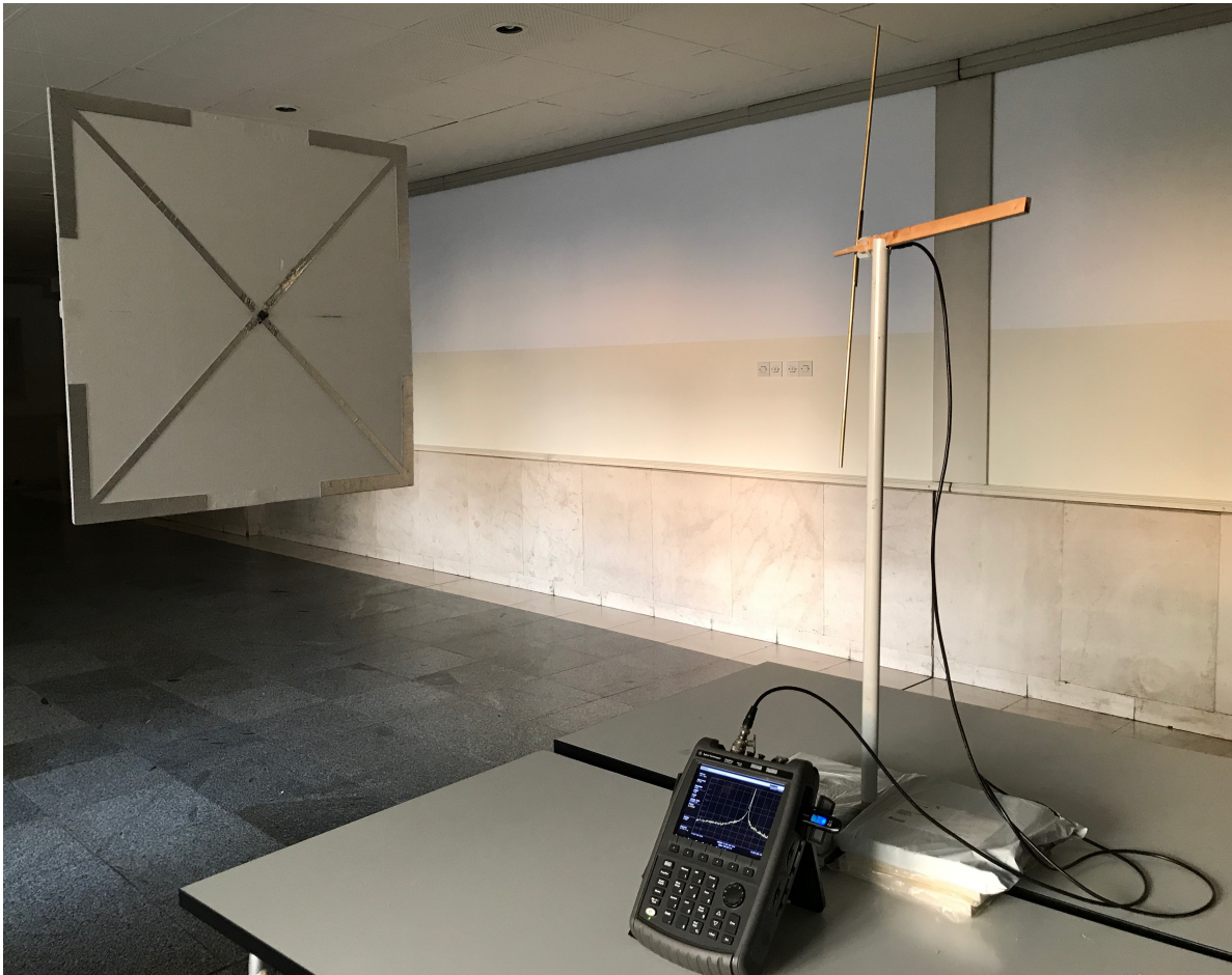
Figure 4.30: Photo of the measurement setup of self-oscillating antenna with crossed capacitively loaded dipoles.
