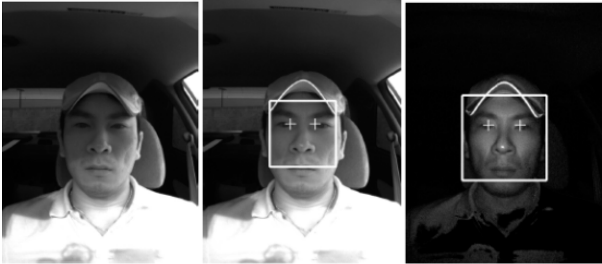
Figure 3.11: The example of the face detection on an ambient frame (left), illuminated frame (middle), and a difference frame (right) [82]
