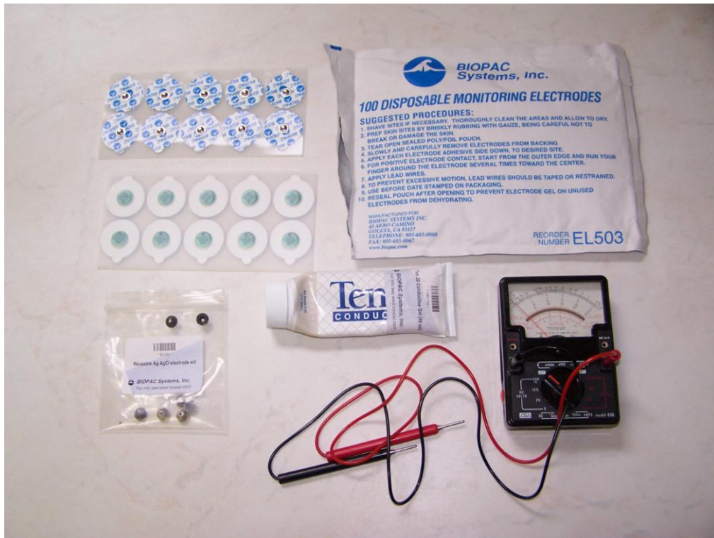
Figure 8.3. Electrodes and accompanying materials used during experiments using the MP35 biopotential amplifier
