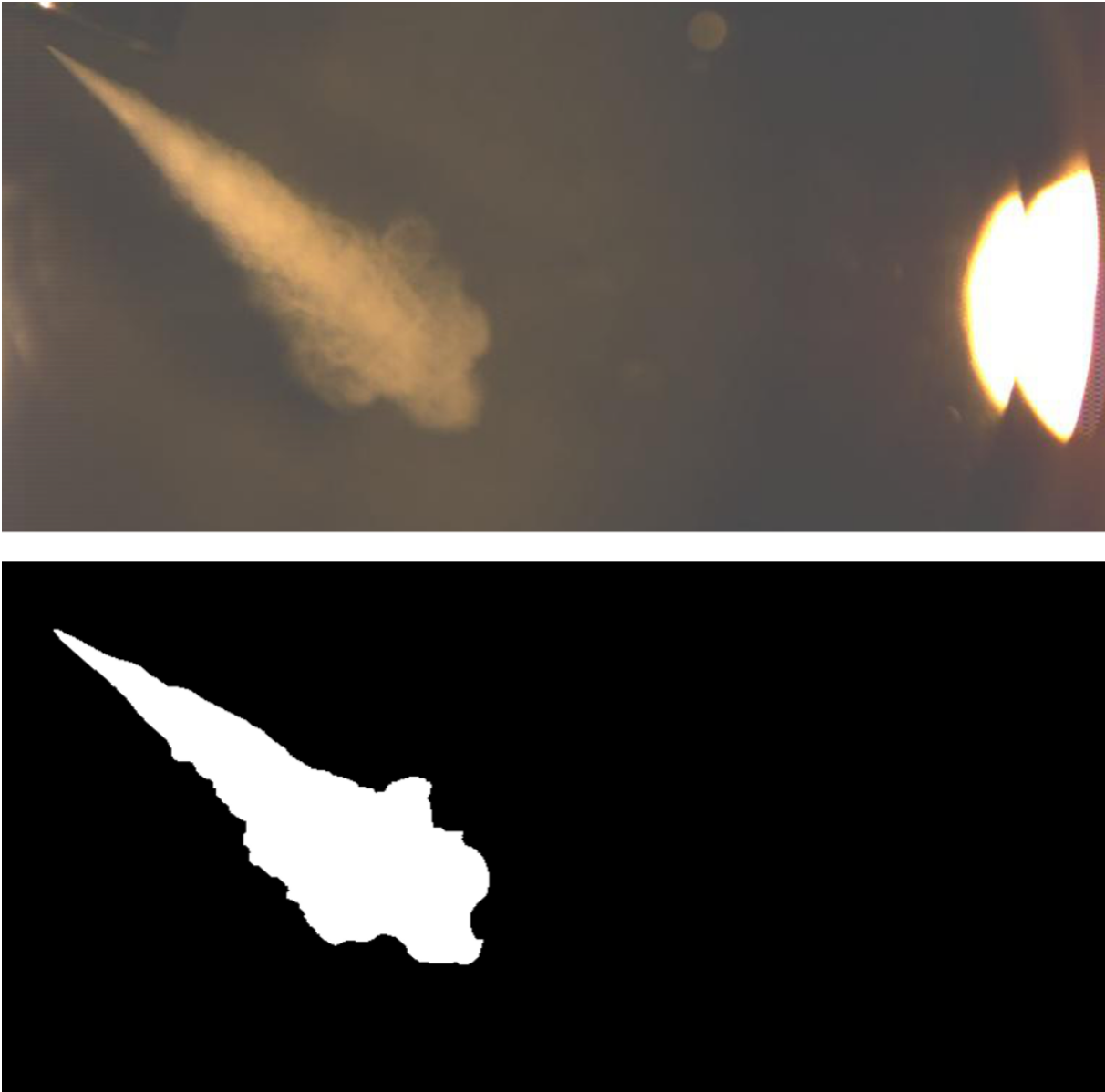
Figure 3.2: Spray image (upper image) and it's corresponding segmentation mask (lower image)
