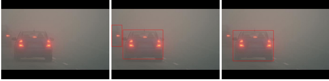
Figure 3.4: Example of an image from the DAWN dataset. On the left is just the image. In the middle is the image with ground truth bounding boxes marked. On the right is the image with detections from a pre-trained detector. Note that the second car is not detected.
