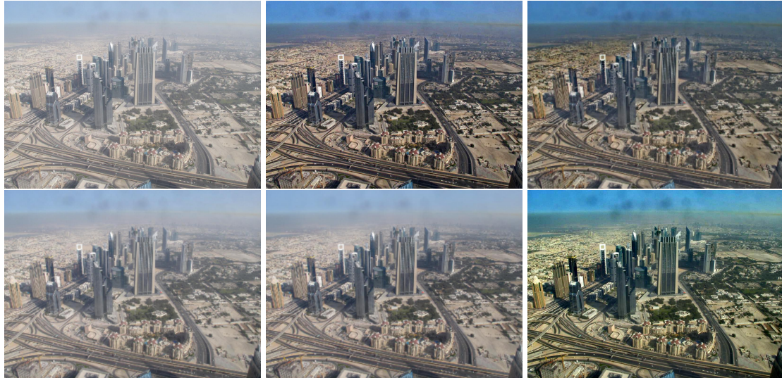
Figure 6.9: Top left is the original image, top middle image dehazed using VarDCP, and top right using Unsupervised DCP. Bottom left is dehazed using FFANet, bottom middle using Dehazeformer, and bottom right using MSCNN. FFANet and Dehazeformer once again do not change the image. The best results come from VarDCP and the Unsupervised DCP.
