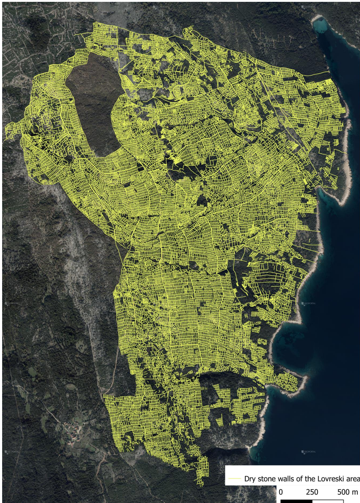
Figure 166. The dry stone walls of the Lovreški area. Over 711.8 km of walls stand in an area of 525 ha, with an overall density of 135 km/km 2 . Vectorisation in GIS by Michela Trevisan and Tanja Kremenić. North is up. Base map DOF 2014 (DGU 2019)
