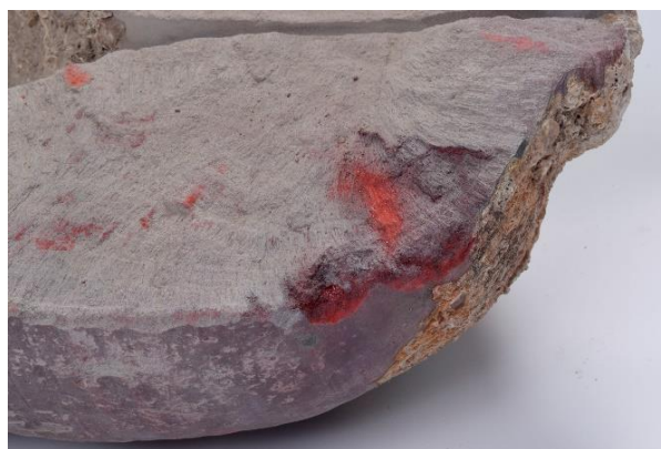
Fig. 9-27. and Fig. 9-28. Grey alteration layer of bell-shaped mercury sulphide, type A (photo: N. Čuk).
