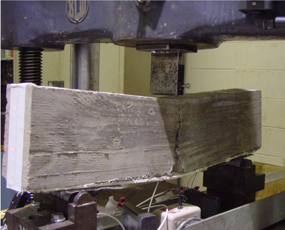
Figure 10.3 Plain concrete beam exposes in the three-point bending experiment under static loading conditions
