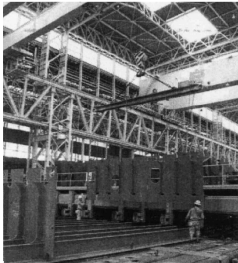
Fig. 3.66. Unit panel and slot construction—sliding on transverses [4]
