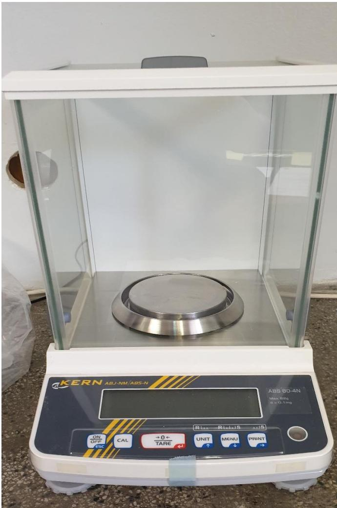
Slika 1. Laboratorijska vaga Analytical balance ABS-N/ABJ-NM
