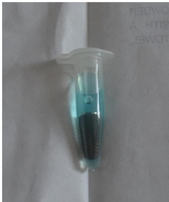
Figure 14. Titanium dental implant immersed in 0.2% chlorhexidine (PC group).
