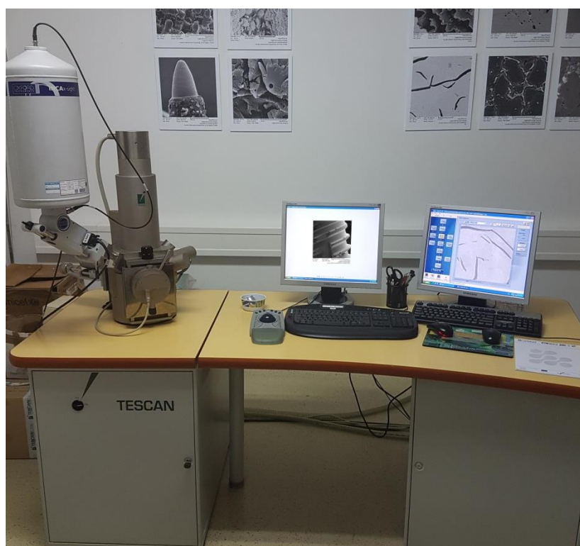
Figure 19. Scanning Electron Microscope (Vega, Brno, Czech Republic).
