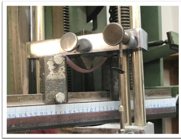
Figure 3. An undamaged polyamide specimen (Vertex ThersmoSens) with loading within the end limits of the possible movement of the penetrant
